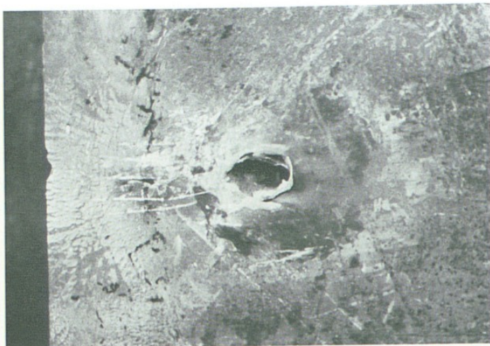
Diagram showing the piercing of an armour plate inclined at 60 deg., by means of an ENERGA grenade
