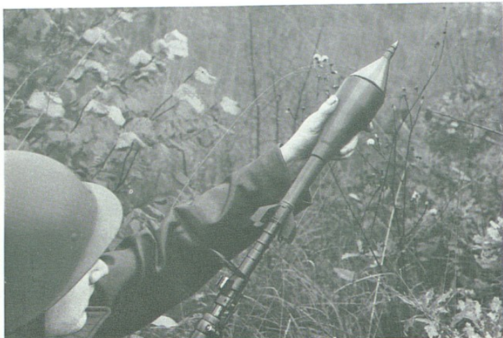
Fitting the grenade on to the launcher
